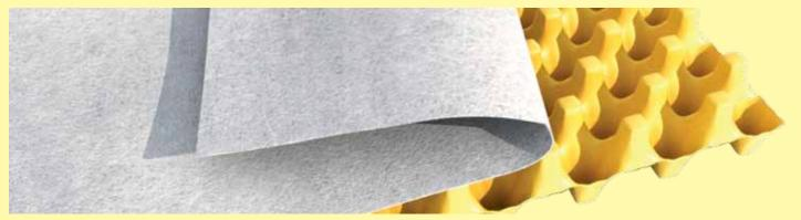
ISOCOR is a drainage geocomposite consisting of a thermoformed, symmetrical, waterproofed, non-compressible HDPE geospacer, thickness 8, 10 16, 20 or 40 mm, sticked to an ASQUAL certified geotextile on one side.
