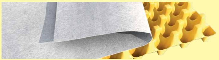
ISOCOR is a drainage geocomposite consisting of a thermoformed, symmetrical, waterproofed, non-compressible HDPE geospacer, thickness 8, 10 or 16 mm, attached to an ASQUAL certified geotextile on one side. ISOCOR performs four main functions: Filtration / Drainage on one side / Air gap along the wall / Waterproofed structure allowing the concrete to be sprayed or poured directly (formwork).
